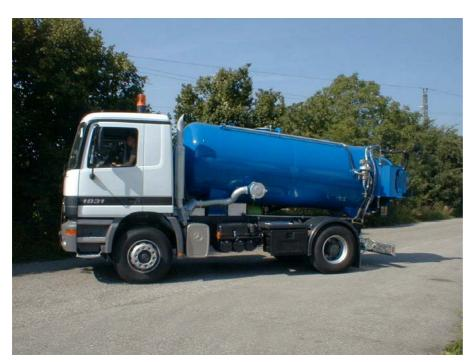
Modern sewer cleaning truck with a tank of 8 m³ and a strong high pressure pump with pressure lubrication system.
