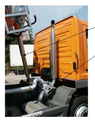
Strong lifting cylinder for tipping the tank, firmly assembled on the vehicle chassis.
