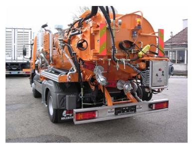
One person can operate our vehicle. All functions can be switched and controlled from the rear of the vehicle.
