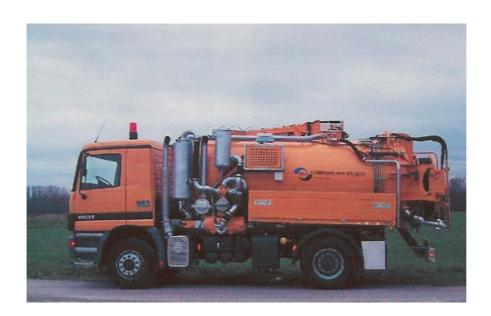
Modern combined sewer cleaning truck with a tank volume of 10m³, strong Highpressure - and Vacuum - Pump.
